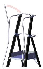
Step 2: Once inside, swing the crossbar back down and into the hooked bracket.
