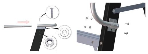
**Step 2**: Fasten top in place with 6x35 mm bolts, 6x13 mm washers, and M6 nuts.
